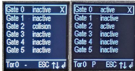
Figure 9-2 Gate inactive, collision / Gate active
