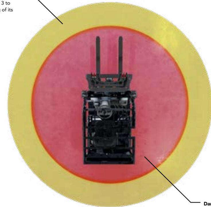
**Danger zone** offers a variable detection range from 3 to 15 meters depending of its configuration.
