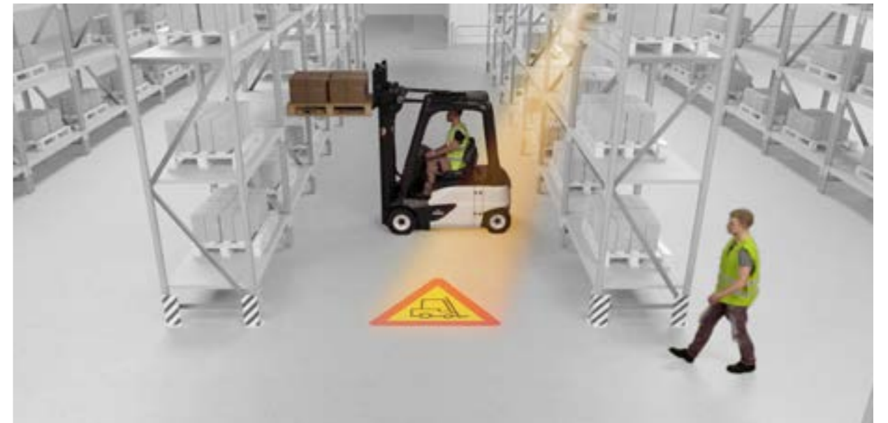
NAS (Narrow aisle system) solution with projection light signals.
