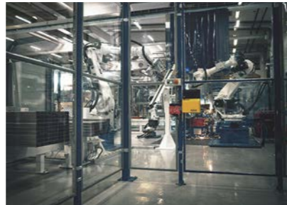
POLYCARBONATE PANELS Gives good overview and protects against fluids and small particles.
