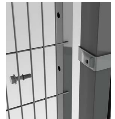
SMART FIX BRACKET Fixed in position with a bolt from the backside of the bracket. Move the bolt to the side position to create a corner.
