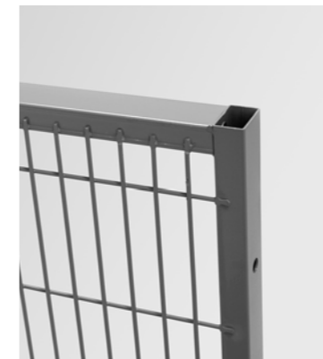
ST30 MESH PANEL The ST30 mesh panel has a classic look with the mesh size of 20x100 mm fixed to a 30x20 mm frame. Available in three standard heights, 1,250, 2,050 and 2,350 mm in up to 8 widths.
