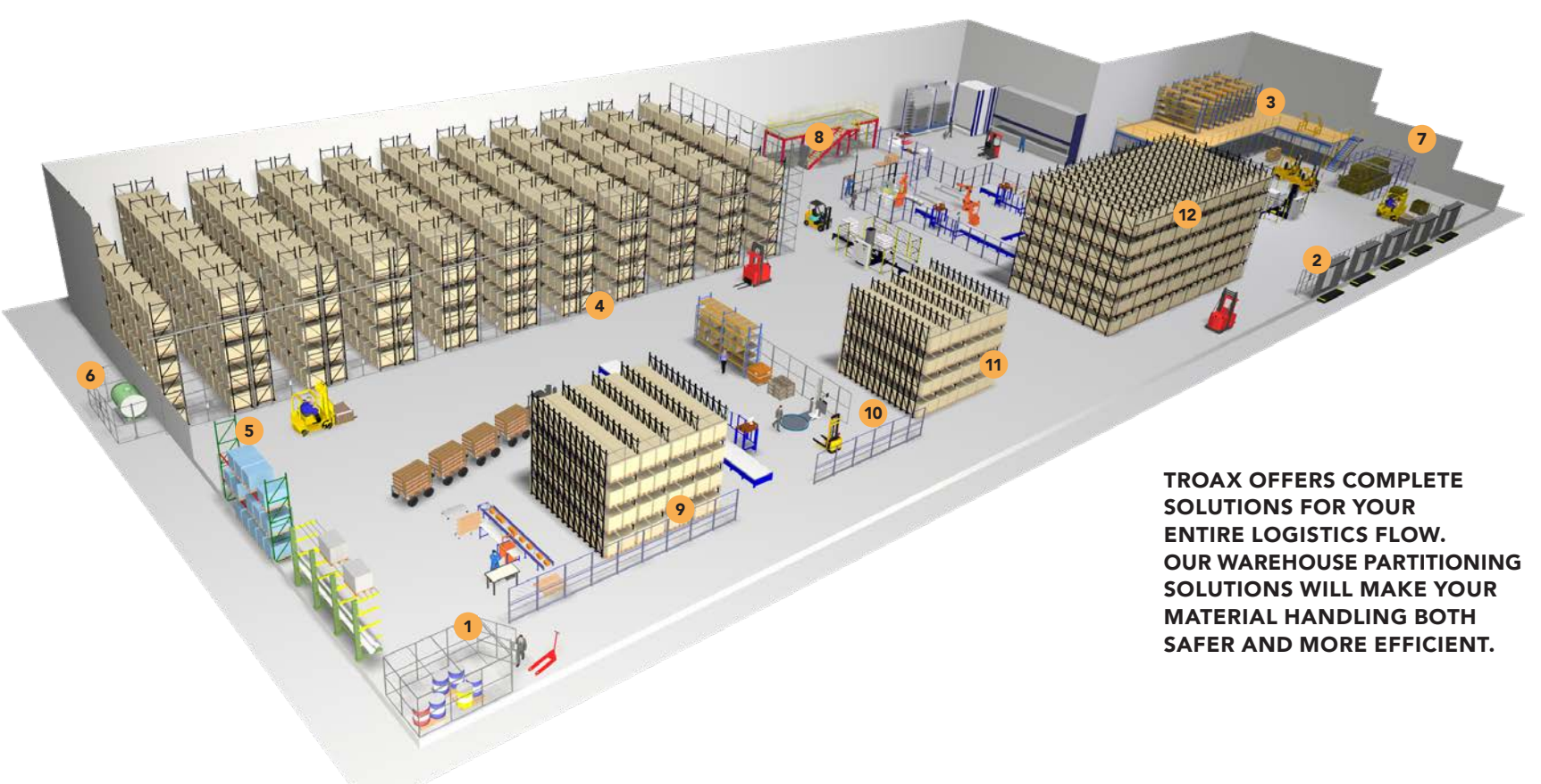
3 MEZZANINE GUARD The Mezzanine system with posts, panels, kick plates and guard rail protects both people and loose objects from falling down.
