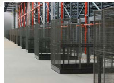
10 TRUCK AISLES The Partitioning System allows warehouse trucks to come through without compromising the safety of personnel or goods.
