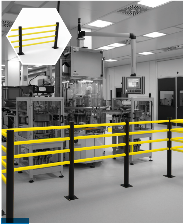
At 22.5° Impact, 4.6 km/h (2,86 mph) and 3.150 kg (6945 lbs) on a C20/25 concrete floor and max. force to bolt at 13 kN.
